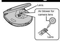
Open the lid and clean the lens as shown in the figure. Use a cotton swab to gently wipe off any finger-prints.
