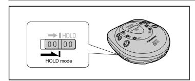
This function causes the unit to ignore short, accidental button presses. (The disc lid can still be opened and closed.)
